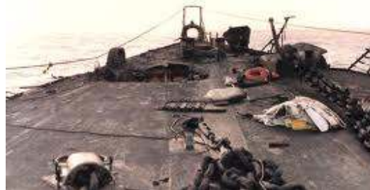
View from the forward MG sets. Bow anchor chain and port lifelines are missing.
